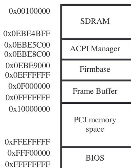
The “Frame Buffer” cannot be accessed directly, this address space is left unused in the system; above table includes a 16Mb “Frame buffer”(can vary from 2- 128Mb)
