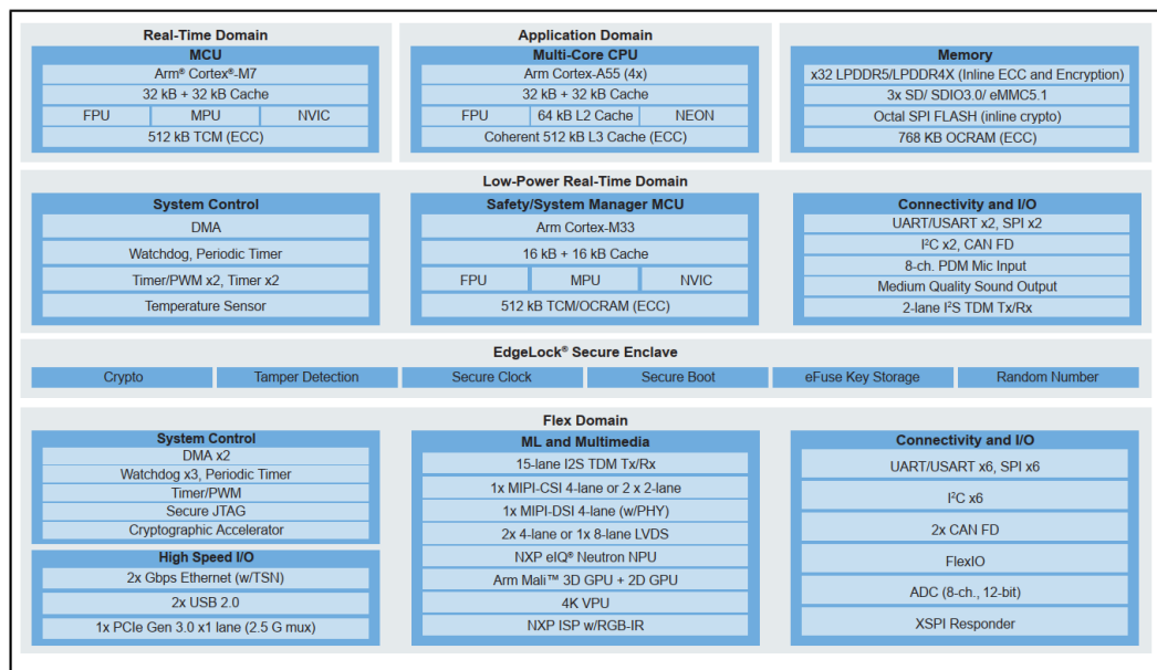
Figure 2 i.MX 952 Block Diagram
